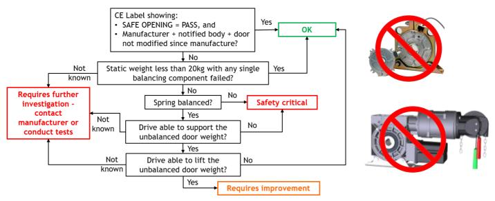
If switching to manual mode with a failed spring would cause the door to fall-back catastrophically, the door must be classified as safety critical. Where a safety brake manufacturer requires the use of a stop switch, but it is not connected, this would be classified as requiring improvement.
