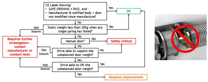
If switching to manual mode with a failed spring would cause the door to fall-back catastrophically, the door must be classified as safety critical.
