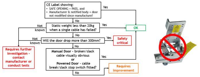
Where a jamming device manufacturer requires the use of a stop switch, but it is not fitted or connected, the door would be classified as requiring improvement.
